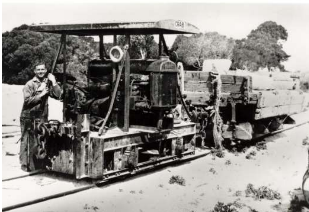
MILITARY RAILWAY – Crab - date unknown. Photo of Crab (transverse mounted engine) towing wagon No 1 and "Curly" Masters (driver). The locomotive Crab (so
